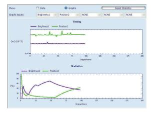
The statistics panel displays all the information about inspection results and execution time. Data can be shown also in a graph.
