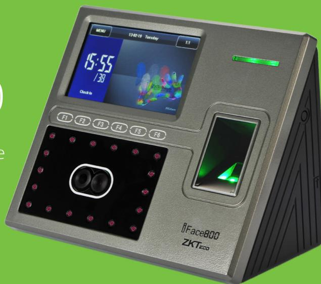
Using the latest ZK platform and algorithms, iFace800 can hold up to 1,200 face templates and 2,000 fingerprint templates. Supporting multiple authentication methods including face recognition, fingerprint, password, RFID card (and combinations), the iFace800 is ready for integration into the most demanding applications. Communication options include serial/RS485, Ethernet, USB host, and optional Wi-Fi or GPRS. An available 2000 mA battery allows system operation during loss of power events.
